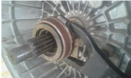
Gambar 5. Pemasangan *Release Fork* Dan *Release Bearing*
