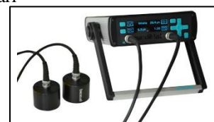
Gambar 2. Alat Ultrasonic Pulse Velocity (UPV) (Sumber: Manual Book Proceq,2017)
