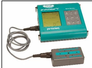
Gambar 7. Alat Rebar Locator (Sumber : Manual Book Proceq)
