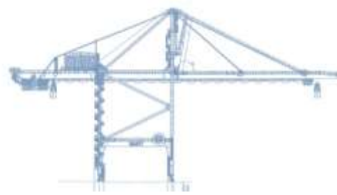
Gambar 2. Tampak samping Rail Mounted Quay Crane
