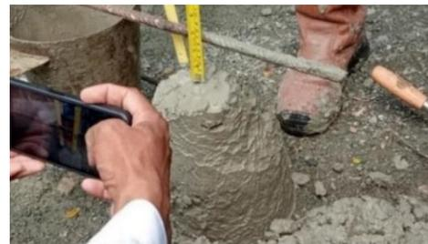
**Gambar 11.** Slump Test
