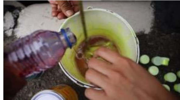
Gambar 5. Proses pencampuran larutan marka glow in the dark
