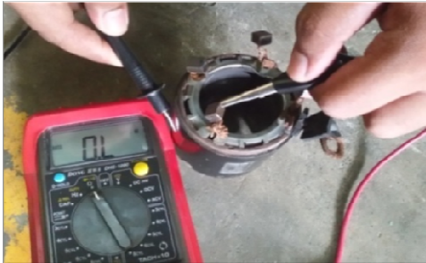
Gambar 9 Periksa Hubungan Massa Field Coil
