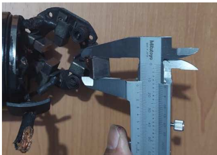
Gambar 10 Pengukuran Carbon Brush
