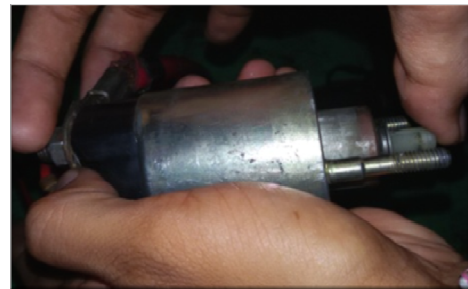
Gambar 12 Test Penekanan Plunger
