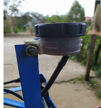
Gambar11 Pemasangan reservoir tank
