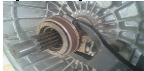
Gambar3 Pemasangan release bearing & release fork
